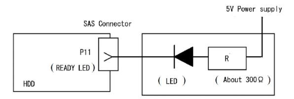
Figure 4.11 Recommended external circuit for Ready LED output
